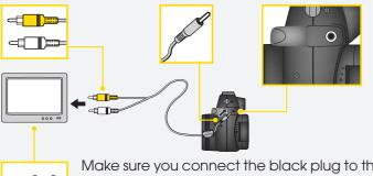
Make sure you connect the black plug to the camera, and the yellow plug to the television Video-in socket, and the white plug to the television Audio-
